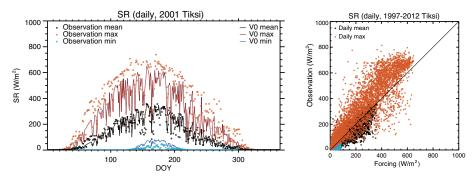
Figure 3. Comparison between level 0 short-wave radiation and observed values. Example shows 1-year time series of daily mean, minima, and maxima during 2001 (left), and scatter plot for all daily data (right) at Tiksi.
