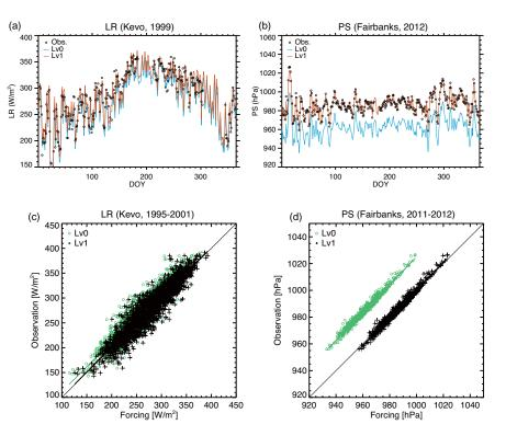
**Figure 6.** Comparison of GTMIP forcing data and observed values for (a) long-wave radiation (LR) of Kevo (in 1999), and (b) surface pressure (PS) of Fairbanks (in 2011) on a daily basis. Level 0 data are shown in blue and level 1 data in red. Correlation between the forcing data sets and observed values for these examples are also shown for (c) LR of Kevo (in 1995–2001), and (d) PS of Fairbanks (in 2011–2012). Level 0 data are shown in green and level 1 data in black.
